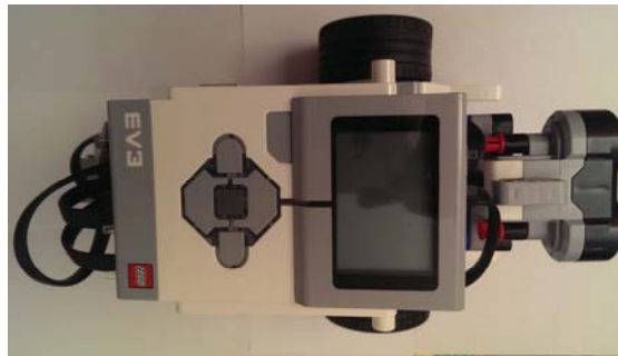
Figure 2. The ultrasonic sensor mounted
